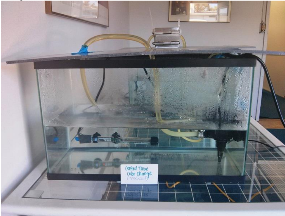
Figure 4. Close-up photo showing aquarium heater, pump, pvc tubing, and halbach magnet.
