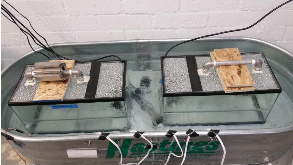
Figure 10. Two tanks both spiked with pond water sit in a water bath held around 94F. The tank on the left circulates water through a 4-link halbach magnet bracelet. The tank on the right has no treatment.
