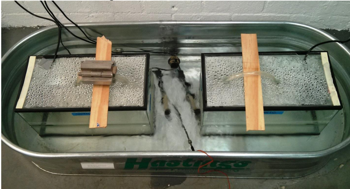
Figure 7. Two 10-gallon tanks sit in a water bath. The tank with magnetic treatment is on the left. The one on the right has no treatment.
