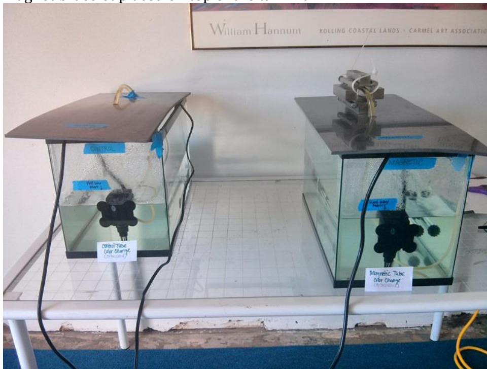
Figure 3. Photo of HPC testing set up. The tank is on the left houses circulating untreated water. The tank on the right houses water passing through a 4-link halbach magnet bracelet placed on top of the tank lid.
